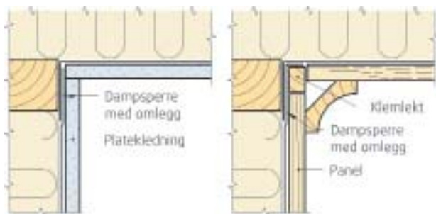
Klemmeprinsipper for dampsperre
